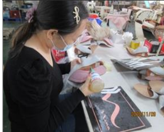
External photo(s) of the production unit(s) 7-6 Gluing worker was wearing medical mask rather than active carbon mask and not wearing the provid.JPG
